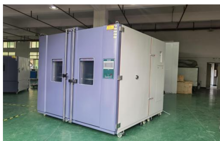
3.6 m3 constant temperature humidity laboratory
